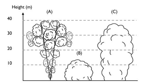
(A) This plume is narrow at the ground level and expands at higher levels; it can be detected readily at these levels. (B) This fire is slow to develop; the temperature of the plume cools around 10m to 15m causing it to stratify at this level. (C) This plume develops at lower levels and doesn't cool until it reaches higher elevations. Due to the high temperature, its size is equal from floor to ceiling.
