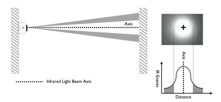
The transmitted beam of Infrared is a cone of light where the intensity or energy of IR light reduces as a function of distance from the axis, as shown on the graph.
