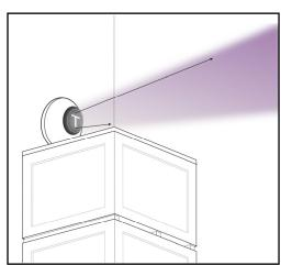
There must be a permanent clear line of sight between the Transmitter and the Receiver or Reflector.
