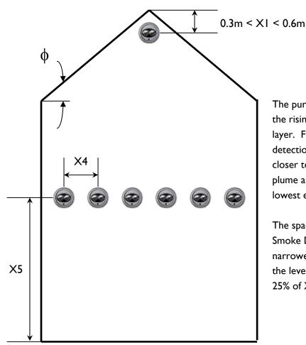
The purpose of this approach is to detect the rising plume rather than the smoke layer. For this approach, supplementary detection is used; OBSDs are mounted closer to ensure they intersect the rising plume and are installed at a level below the lowest expected stratification level.
