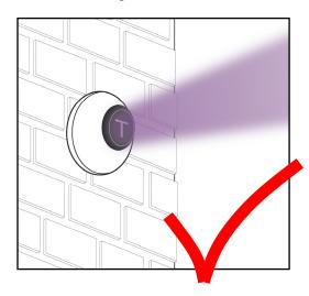
Mount the OBSD on a stable mounting surface such as brick, concrete, a sturdy load-bearing wall, support column, structural beam or other surface that is not expected to experience vibration or movement over time.
