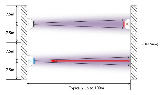
Hence an Optical Beam Smoke Detector can protect a wide area up to: 1,500 m<sup>2</sup>
