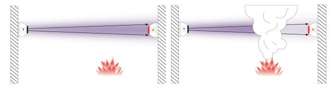
The Optical Beam Smoke Detector (OBSD) works on the principle of light obscuration. The photosensitive element of the OBSD detects IR light produced by the Transmitter in a normal condition. The Receiver is calibrated to a preset sensitivity level based on a percentage of total obscuration.
