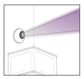
Any object in the infrared light beam path could cause a reduction in signal and ultimately may prevent the system from operating correctly.
