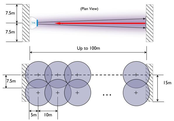
Optical Beam and Point-Type Smoke Detectors have their own applications. Fewer Devices = Lower Installation and Maintenance Costs.
