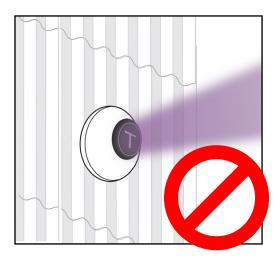
**DO NOT MOUNT** the Optical Beam Smoke Detector on corrugated metal walls, sheet metal walls, external building sheathing, external siding, suspended ceilings, steel web trusses, rafters, non-structural beam, joists or other such surfaces.
